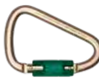
Steel Carabiner 5005 Length: 4.88" (124mm), Opening: .94" (24mm), Breaking Strength: 9,218 lbs. (41kN)
