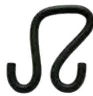
Bucket Hook 5358 Size: 5/8" Material: PVC Fits Bucket Size: 3" lip Breaking Strength: 100 lbs. *Model 5058 available for standard lip baskets*
