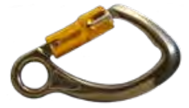
Aluminum Carabiner w/Eye 5005SAE Length: 5 1 / 4 " (133mm), Opening: .71" (18mm), Breaking Strength: 5,732 lbs. (25.5kN)
