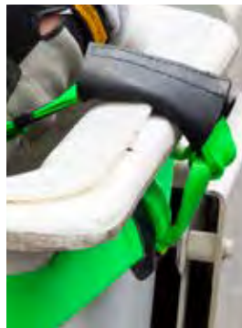
10,000 lb. nylon straps attach to bucket with a ratchet buckle.
