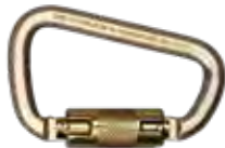
Steel Carabiner 5005T Length: 4.38" (111.3mm), Opening: .94 (24mm), Breaking Strength: 9,218 lbs. (41kN)
