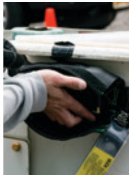
The 10,000lb nylon straps attach to the bucket with a ratchet buckle.
