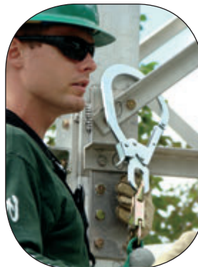
Tie Back Snaps can attach to the ring of the ANSI rated Big BuckSnaps™, and hooked directly over tower lattice. Note: ComboYard™ becomes a 6' dual shock absorbing lanyard when Big BuckSnaps™ are added.
