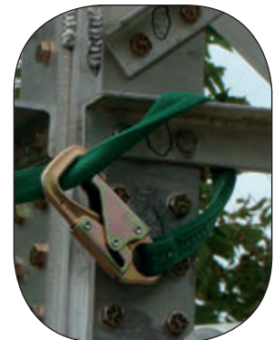
Tie Back Snaps can be attached back to the lanyard. This allows climber to continue to use the lanyard in the event of larger attachment points.
