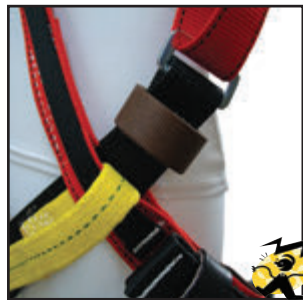
E = LEFT SIDE ONLY E1 = RIGHT SIDE ONLY 1 3/4" diameter loop (1" 4-ply nylon) in hip area to attach snap hook. FOR BOTH SIDES USE EE
