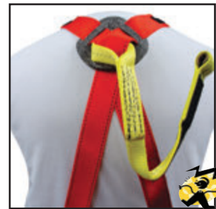
G = 18" extension strap (1" yellow web) that terminates with 3/4" diameter loop for carabiner.
