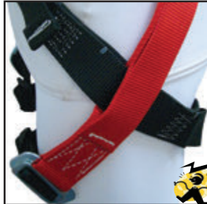
R3 = Type X red upper section, black lower section. No chafes under buckles.
