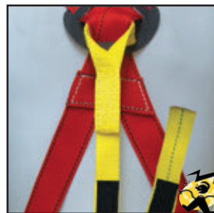
G1 = 18" extension strap (1" yellow web) with a loop (approx. 3" dia.) to half hitch on an energy absorber.
