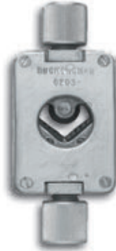
Model 6203 Outside diameter capacity of 1/4" to 1" Maximum handle swing of 3" for work in closely confined places For such applications as cylinder head studs, 'U' bolts, wheel lugs, etc Weighs 1 1/4 lbs.
