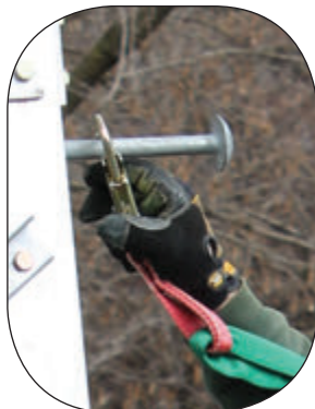
Tie Back Snaps can be used to snap over step bolts. Note: Step Bolts must have a large enough head to prevent snap from sliding off.
