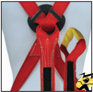
G3 = 18" extension strap (1 3/4" orange web) with wear piece around 3 1/2" diameter loop for attachment of energy absorber.
