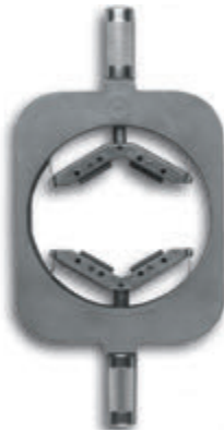
Model 62070 Outside diameter capacity of 4" to 6". Has plain guide die blade which allows dies to pass over keyways and milled flats on threaded parts. Weighs 4 1/2 lbs.
