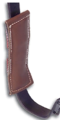
Model 35033 - Climber Footplate The climber footplate attaches easily to any steel or titanium climber. Two plate construction fastened together with two screws. Simply screw the two plates together with the rubber sole down. Standing on the pole was never so comfortable. Instructions packed with footplate. To order replacement screws use part #14. Not for use with aluminum climbers.
