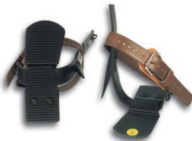
Model 35033 - Climber Footplate The climber footplate attaches easily to any steel or titanium climber. Two plate construction fastened together with two screws. Simply screw the two plates together with the rubber sole down. Standing on the pole was never so comfortable. Instructions packed with footplate. To order replacement screws use part #14. Not for use with aluminum climbers.
