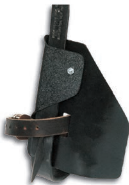
Model 10 - Climber Shield A light weight shield that is ideal for apprentices. Helps prevent gaff puncture wounds when learning to climb. Shield attaches easily with one screw to the climber shank. Slot in shield allows for climber foot strap.
